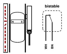
" Installed opposite to indication rail " Cable exit downwards
